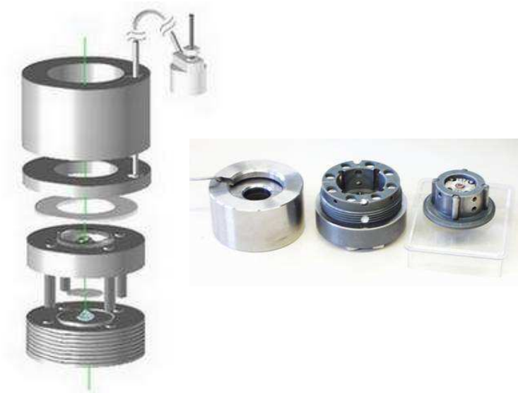
FIGURE 3.3: Sketch of the piston-cylinder BETSA DAC.
