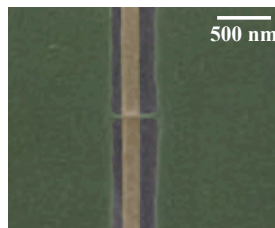
Figure 2.2: Scanning electron micrograph of a QW device consisting of a very narrow channel with a straight metallic strip gate deposited on top.
