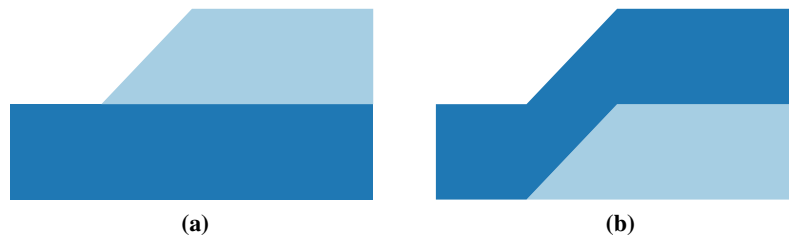
Figure 4.4: Two orderings of two layers on a flat baseline. Case (b) produces a distortion, case (a) is preferred.
