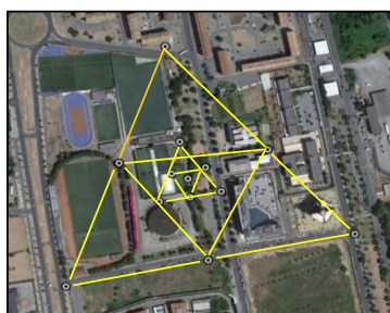
(24 geophones, 10 Hz, inter-space 3 m)
