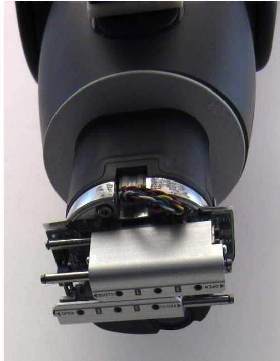
FIGURE 5.5: Sliding bars to which the gripper fingers are mounted.
