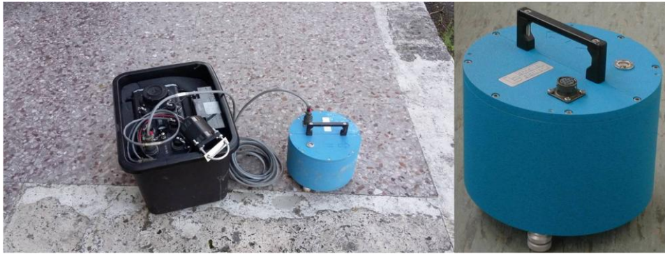
Fig. 12.7 Acquisition system for the Array 2D test
