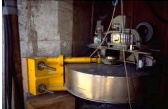
Fig. 11.2 Vibrodyne used by ISMES for the test (1995)
