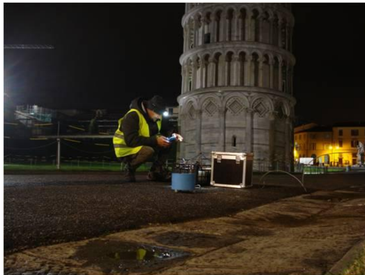
Fig. 12.9 installation of a seismic station close to the Tower
