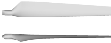
Figure 4.6: CAD rendering of NREL wind turbine blade
