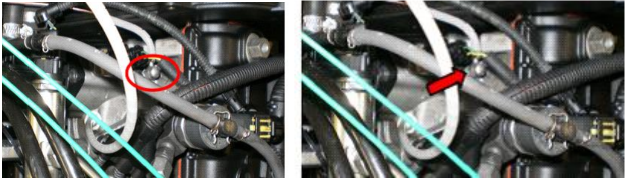
Figure no IV Accelerometer transducer location
