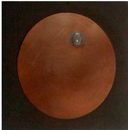
Fig. 45: Photograph showing the realized elliptical patch antenna with the dimensions given in Fig. 93.
