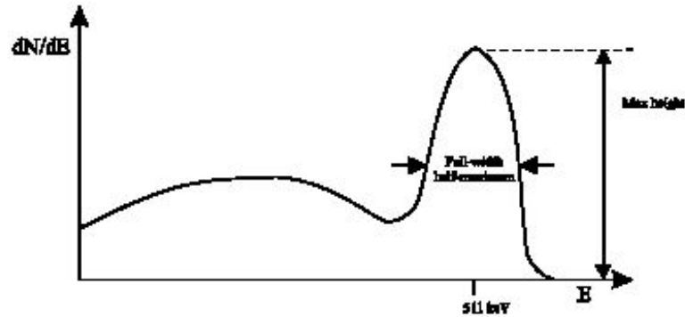
Figure 3.4. Features of a typical energy distribution measured by a scintillation detector system exposed to 511 keV photons ( Badawi [44] ).
