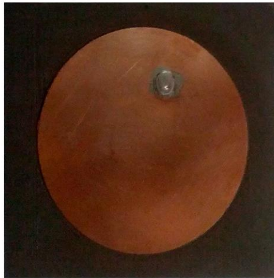
Fig. 98: Photograph showing the realized elliptical patch antenna with the dimensions given in Fig. 93.
