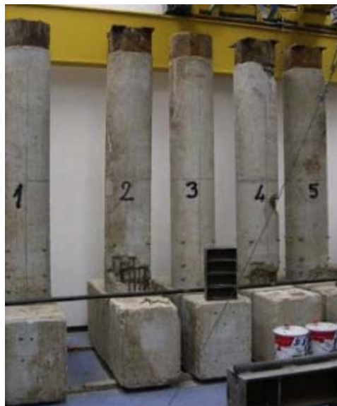
Figure 6.3 Pier Specimen corresponding to the middle pier in the regular bridge
