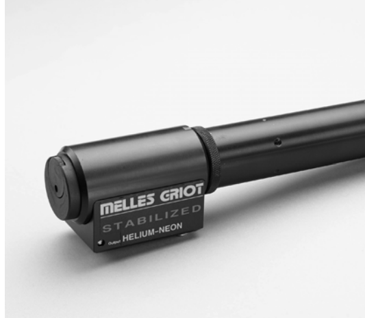
Figure 4.3: picture of the stabilized Helium Neon laser used in the experimental setup
