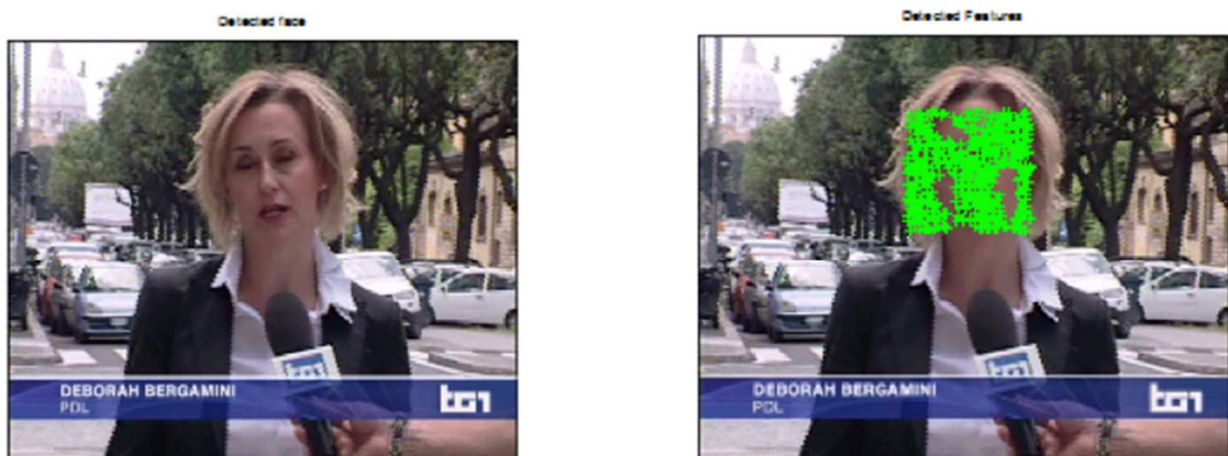
Figure 27 – Case of application of KLT algorithm: On the right the frame with a face with a number of features with overlap of features
