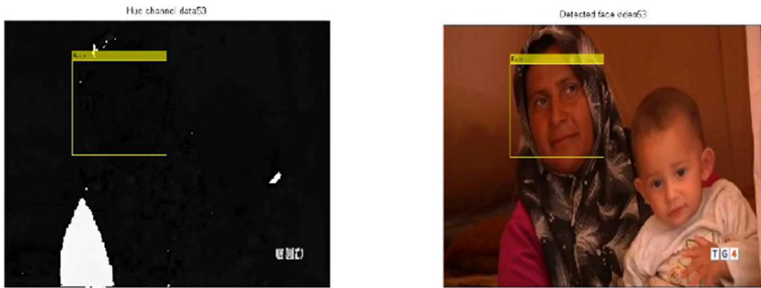
Figure 33 - Map of the hue in which a face in the foreground has a uniform colour from the background
