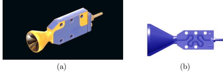
Figure 3.10: External view (a) and designed path (b) of a single channel electron multiplier. Figures from [93].
