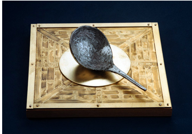
Figure 1.1: Working model of the first instrument known as a compass composed by a magnetic lodestone spoon and a bronze plate. Image from the web.
