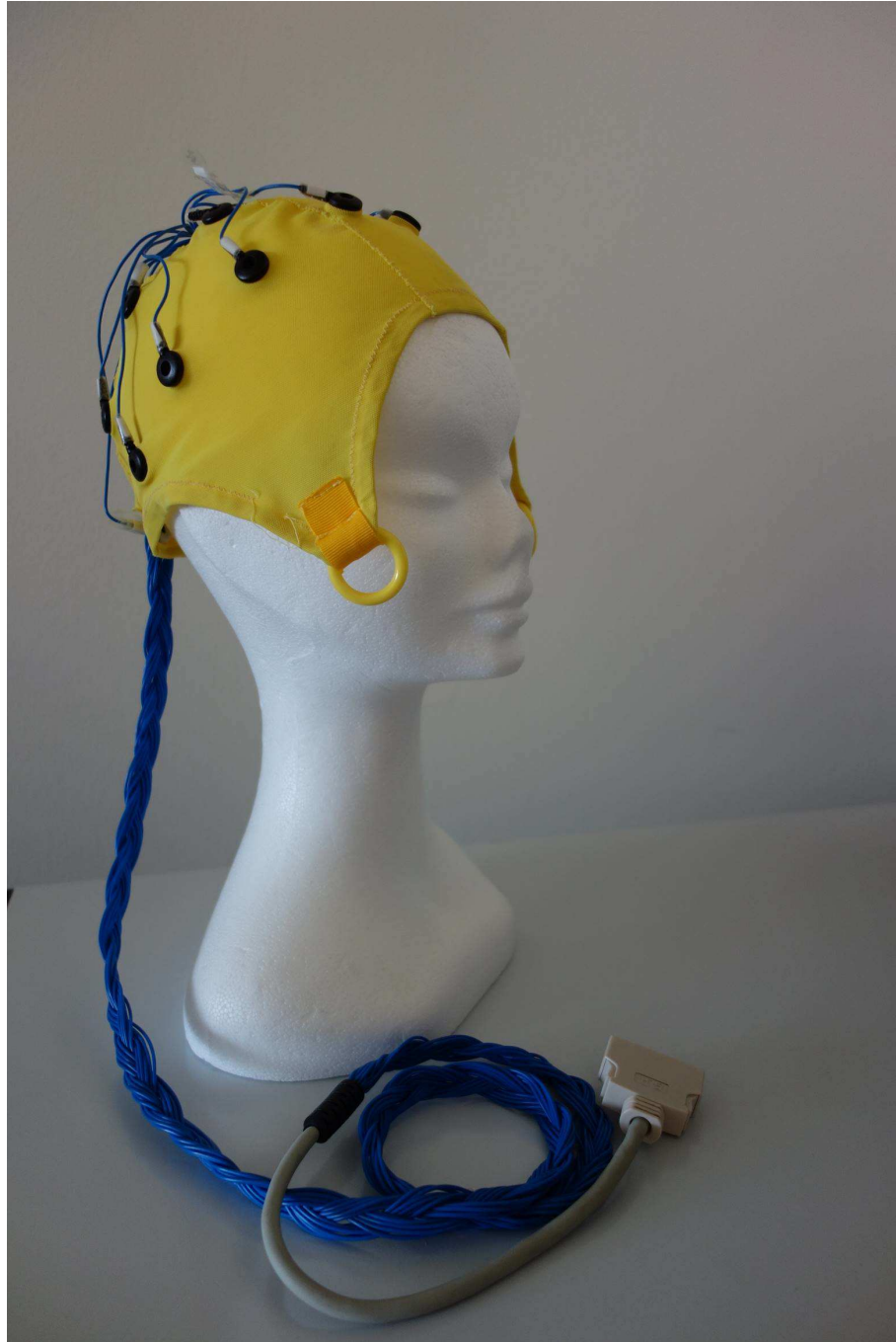
FIGURE 4.2: Headset composed of 19 electrodes used for acquisitions.
