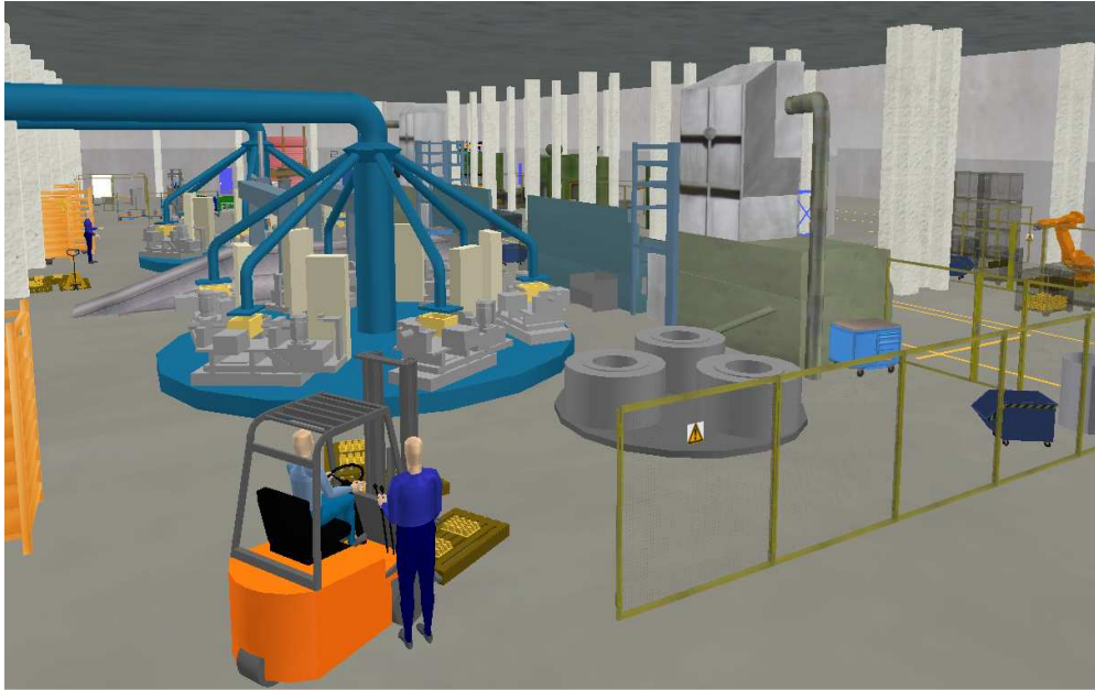
Fig. 12: Example of a Digital Factory model within the IVS_VDT platform (© Fraunhofer IFF)
