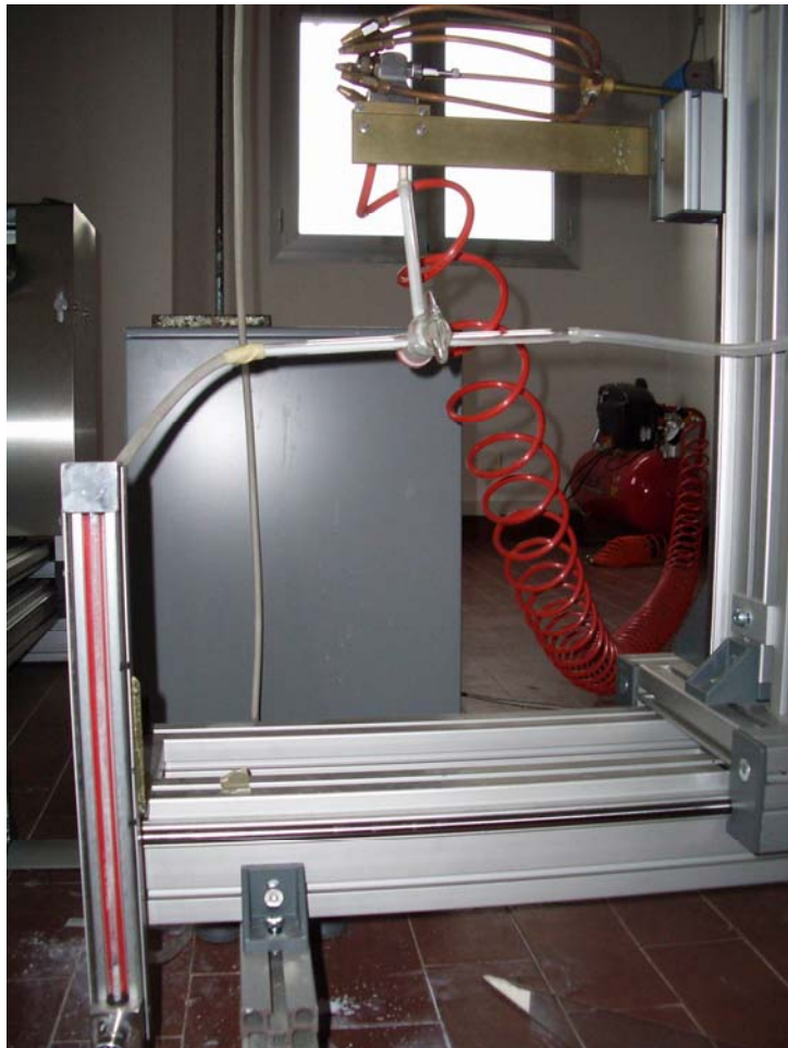
Fig. 3.9 Detail of flowmeter and three way valve.
