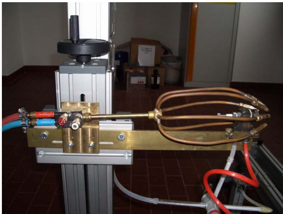
Fig. 3.5 Detail of the Flame spraying equipment with the burning set and atomizing nozzle. Lateral view.
