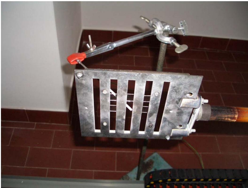
Fig. 3.10 Thermocouple positioning during a deposition onto glass substrate
