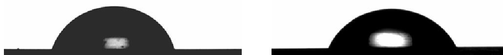
Fig. 5.10 Image of water contact angles on TiO 2 nanoparticles coated PET before and after UV light irradiation.
