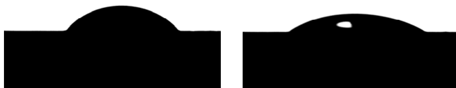
Fig. 5.9 Image of water contact angles on TiO 2 nanoparticles coated glass before and after UV light irradiation.
