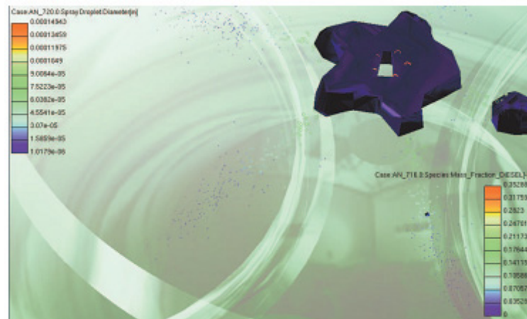
Figure 3.23: Spray droplet diameter- Diesel mass fraction isosurface (0.0065) – TDC
