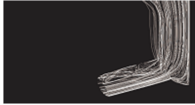
Figure 3.11: 3D injector flow streamlines - 0.315 ms ASOI
