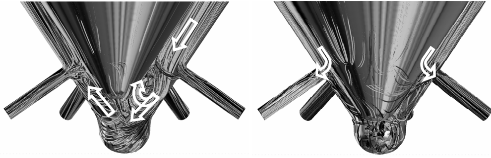
Figure 8.15 (left): Injector1 at full eccentric 1 lift, streamlines
