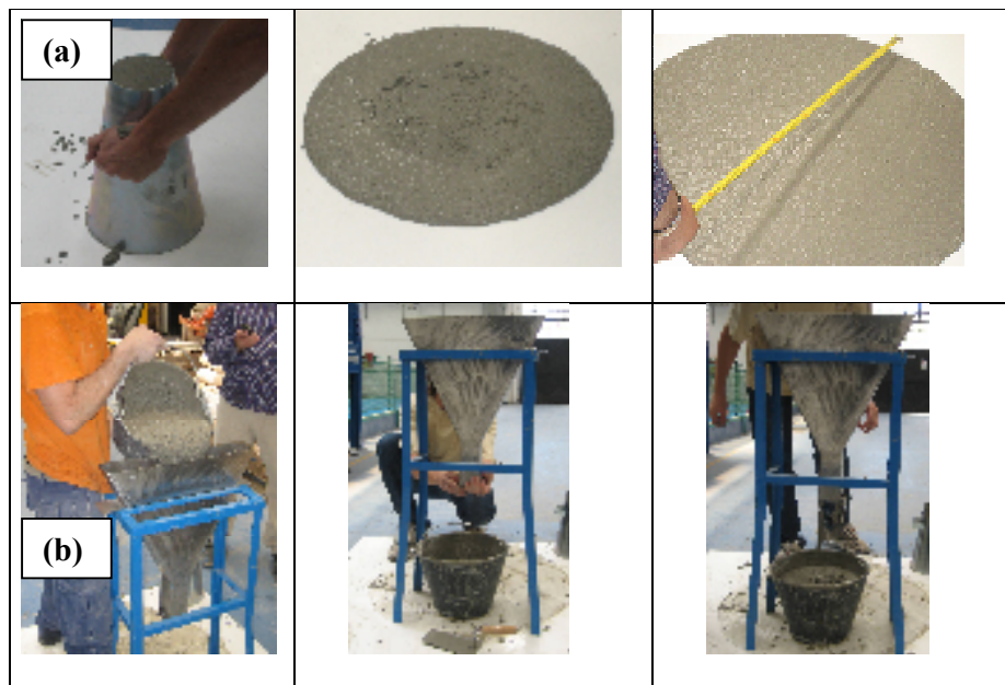
Figure 5. Tests were on fresh material to verify Code UNI 11040 (2003) (a) Slump flow test, (b) V funnel
