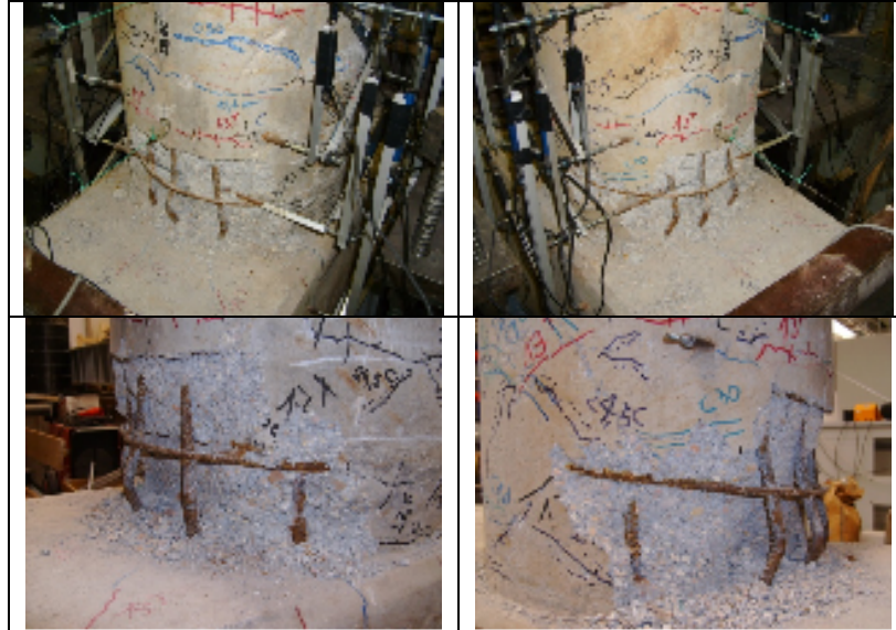
Figure 61 Damages of the specimen 7 at the end of cyclic test
