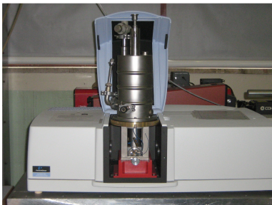
Figure 3.11: PerkinElmer Lambda 950 UV/Vis/NIR spectrophotometer at the ENEA C.R. Frascati.
