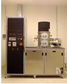
Figure 3.4: GP20 SISTEC-Angelantoni evaporation facility at the ENEA C.R. Frascati.
