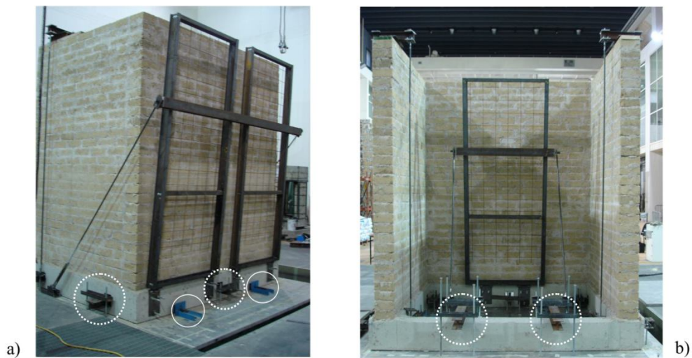
Figure 3.3 View of the specimen with the anchor devices and the retaining structure: UNP 100 steel channel (dotted line) and steel heels (solid line)
