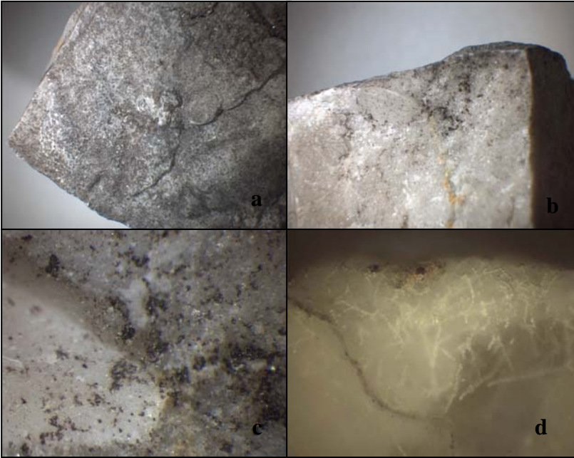
EN5 - Stereomicroscope observations of the surface and of the side fragment (a,b); particular of the surface (c); polished cross section (d)
