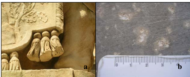
Deterioration phenomena on Bernini's Elephant statue – Area with pits (a); details of a deteriorated part (b)
