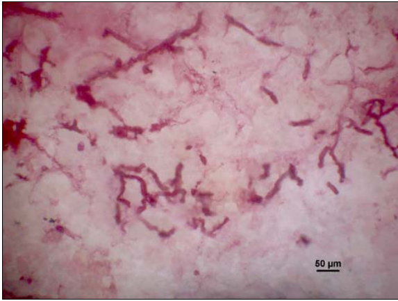
Fig. 5 - Penetration of endolithic microorganisms detected through PAS (Periodic Acid Schiff's reagent) stain techniques.
