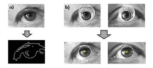
Figure 4.7 – Iris detection. The Sobel operator is applied to detect the edges in the image (a) and a modified Hough transform algorithm is then used to choose the two most voted circumferences among the candidates (b).
