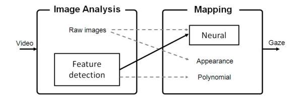
Figure 4.14 – General scheme of a procedure for a view-based REGT system. The dashed arrows indicate the classical view-based techniques. The solid arrow shows the proposed approach, where feature detection is combined with neural mapping to make the system robust to light changes and head movements.
