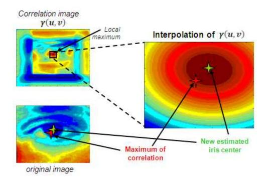
Figure 4.13 – Sub-pixel optimization. The correlation image is interpolated using a mask with a higher spatial resolution. The new local maximum of the interpolated function gives the new position of the iris.
