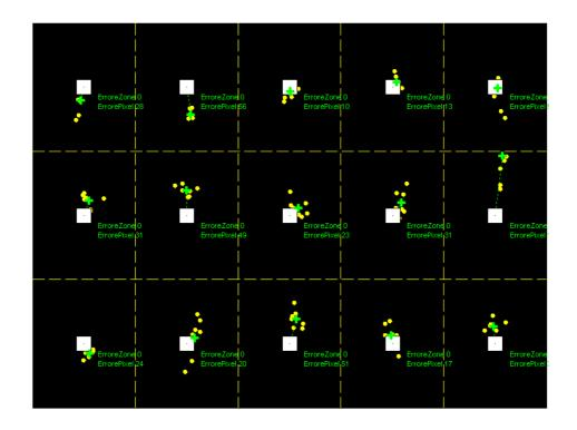
Figure 5.1 – Performance of the gaze tracker on a 15-position interface. The white squares represent the observed points while the dots represent the estimated positions.
