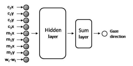
Figure 5.14 - The GRNN used to identify the observed object.
