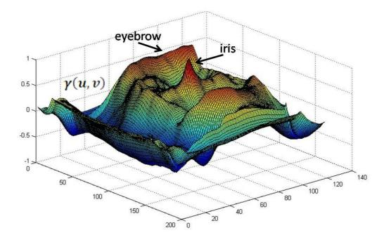
Figure 4.11 – The correlation image. The 3D shape of the surface around the local maximum of the iris is different respect to the other local maxima.
