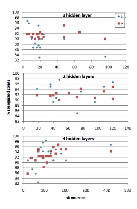
Figure 6.3 - MLP preliminary results. Classification performance as a function of the number of neurons of the MLP net across the different number of hidden layers.
