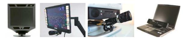
Figure 2.2 – Remote eye-gaze trackers (REGT) as stand-alone solutions, or to be applied to personal computers and laptops. a) MyTobii; b) EyeGaze; c) ERICA; d) EyeTech.
