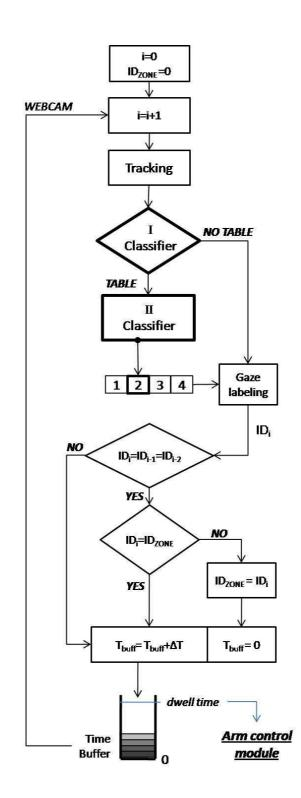
Figure 5.12 - The algorithm of intention prediction through gaze analysis.
