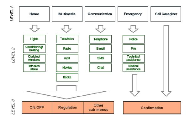
Figure 5.7 – Scheme of the three-level domotic algorithm.
