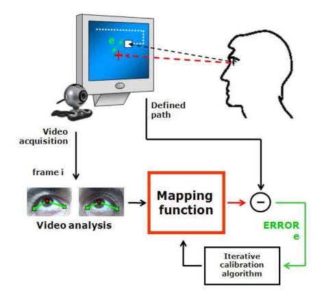
Figure 3.3 – The calibration procedure. While the cursor is moving on the screen on a predefined path, the mapping function calculates the gaze (red arrows). Through an iterative process, the error (depicted in green) between the exact and the estimated position is used to adjust the internal coefficients of the mapping function.
