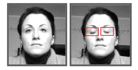
Figure 3.6 – Blink detection can easily serve to detect the location of the eyes by individuating the regions of high movement.
