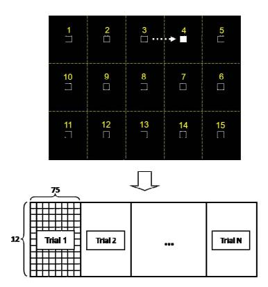
Figure 4.17 – The training procedure. Example with 15 points and 7 frames grabbed per position. The upper panel represents the screen with the 15 positions that the user is asked to look at during one trial. For each position, 5 of the 7 video frames are processed and analyzed to build up a 75 columns (5x15) matrix, each column representing a 12 parameters vector. The remaining 2 frames per position will be used to validate the algorithm.
