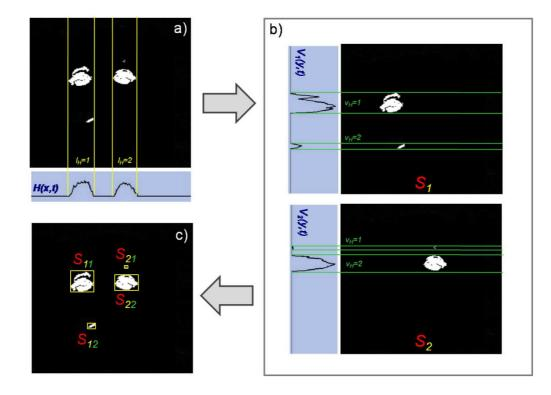
Figure 4.5 – Clustering process. a) The image is clustered through projecting blobs on x-axis. b) The same labeling process, is applied on y direction to each sub-images resulting from the previous step. c) Step a) and b) are merged to finalize the clustering of the blobs.
