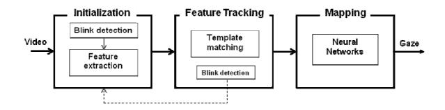
Figure 4.1 - Proposed eye-gaze tracking procedure.
