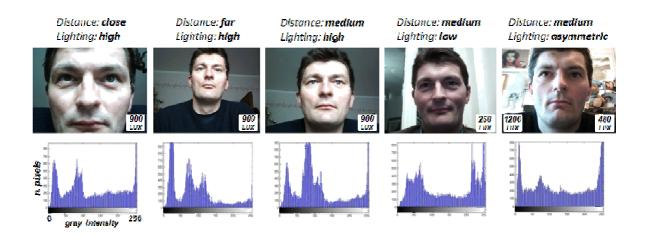
Figure 6.1 – Illumination and distance modifications. Five different combinations of illumination and distance from the camera have been tested for the algorithm. Below each picture, the histogram representation of the luminance distribution is depicted.
