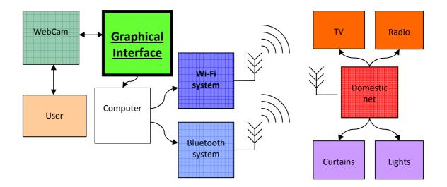
Figure 5.6 – Scheme of a domotic system.
