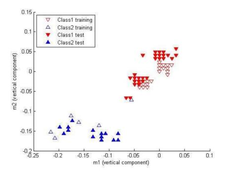
Figure 5.13 - First gaze classification: distribution of the parameters. The upward-pointing triangles represent gazes away from the table, while the downward-pointing triangles indicate that the user is looking to the objects.
