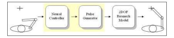
Figure 5.15 - The structure of the bio-inspired arm controller.
