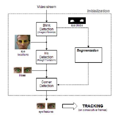
Figure 4.3 - The initialization procedure. Three consecutive steps have been adopted and integrated in the initialization procedure: blink detection, iris detection and corner detection. This procedure allows the system to extract the feature templates to be used by the subsequent tracking procedure.
