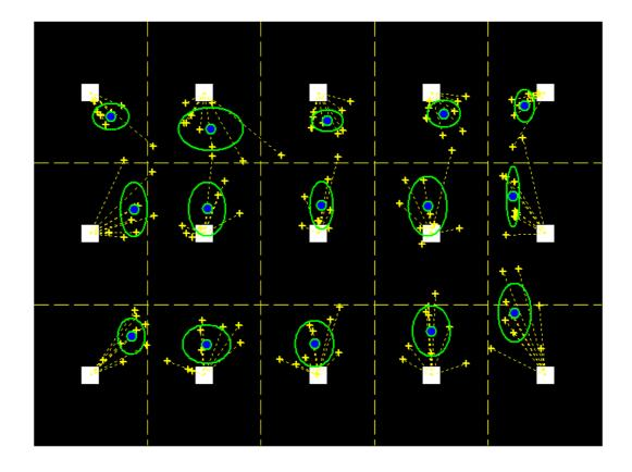
Figure 6.5 - Accuracy evaluation. White squares represent the observed positions. Crosses correspond to the estimated values (1 for each test trial). Small circles represent mean values among the trials, while the ellipses stand for the standard deviations in x and y direction.
