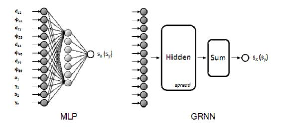
Figure 4.16 – Network architectures. The multilayer perceptron (MLP, left) and the general regression network (GRNN, right), both with a 12 input layer and a single output neuron for the calculation of either the x or the y coordinate of the observed point on the screen.
