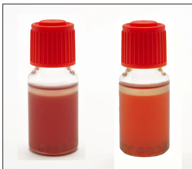
Figure 7: Change of colour of MBS vials for the detection of E. coli with lactose negative Enterobacteria without acidification of medium
