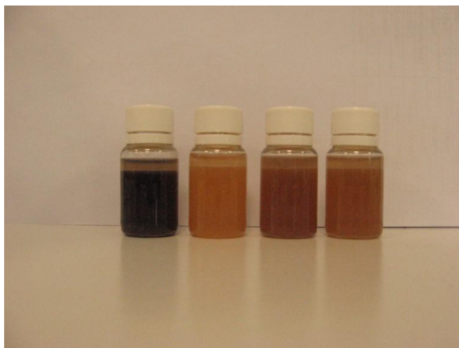
Figure 18: TVC; vials incubated in the thermostat without packaging after 3 months. From left to right: control, 10^{-3} , 10^{-6} , and 10^{-9}
