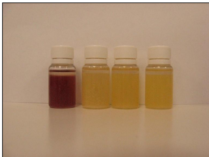
Figure 22: New COLI reagent after 8 weeks; vials incubated in the thermostat in a metal envelope. From left to right: control 10^{-3} , 10^{-6} , 10^{-9}
