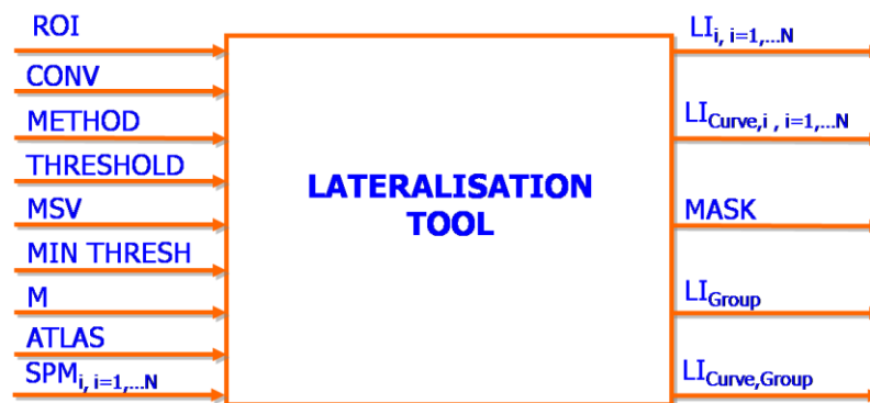
Figure 3.22 – Black box representation of the tool implemented to determine the lateralisation index.
