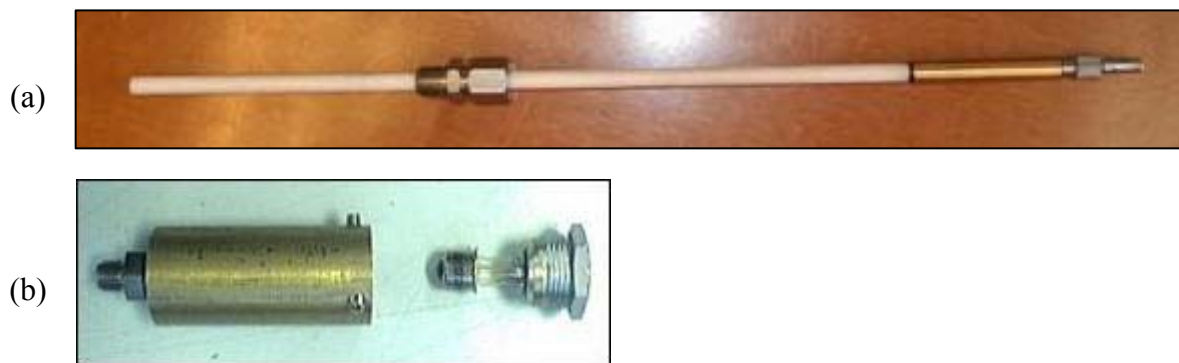
Fig. VII-1: Component parts of ODC technique: monomodal sapphire head with alumina protection (a) and photodiode connection with optical fiber (b).
