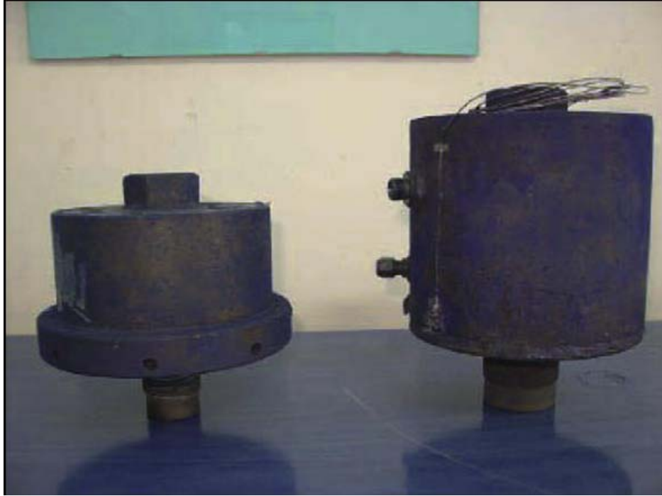
Fig. III-1: Helmholtz resonators mounted in the Siemens annular combustor rig ([I-32], [II-34] § 5).
