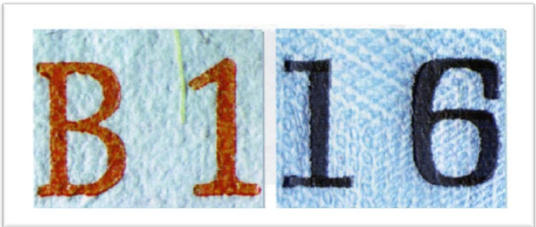
Figure 2.6 – Typical letterpress characteristics are dot fringes (left) and/or the relief-like impression in the paper (right).
