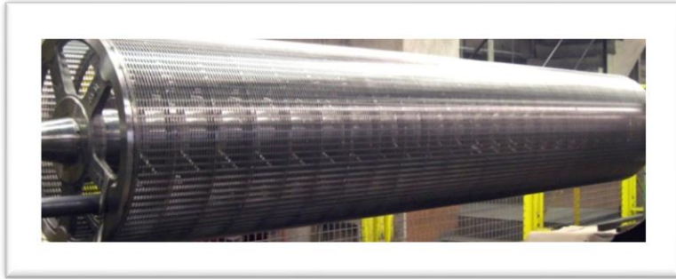
Figure 2.1 – Modern dandy roll example used for printing watermarks on paper in light way.
