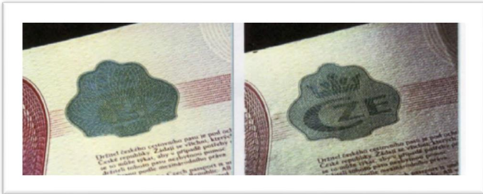
Figure 2.4 – The use of a corresponding design in association with intaglio print allows the printing and, as a result, the detection of a picture or text, which would otherwise remain hidden (latent image/ tilt effect in a Czech Republic passport).
