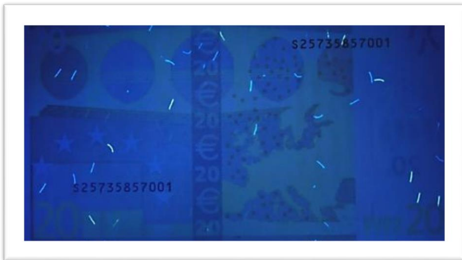
Figure 1.6 – Banknote image acquired under ultraviolet illumination. It is simple to notice the random security metallic fibres distribution inside the image.
