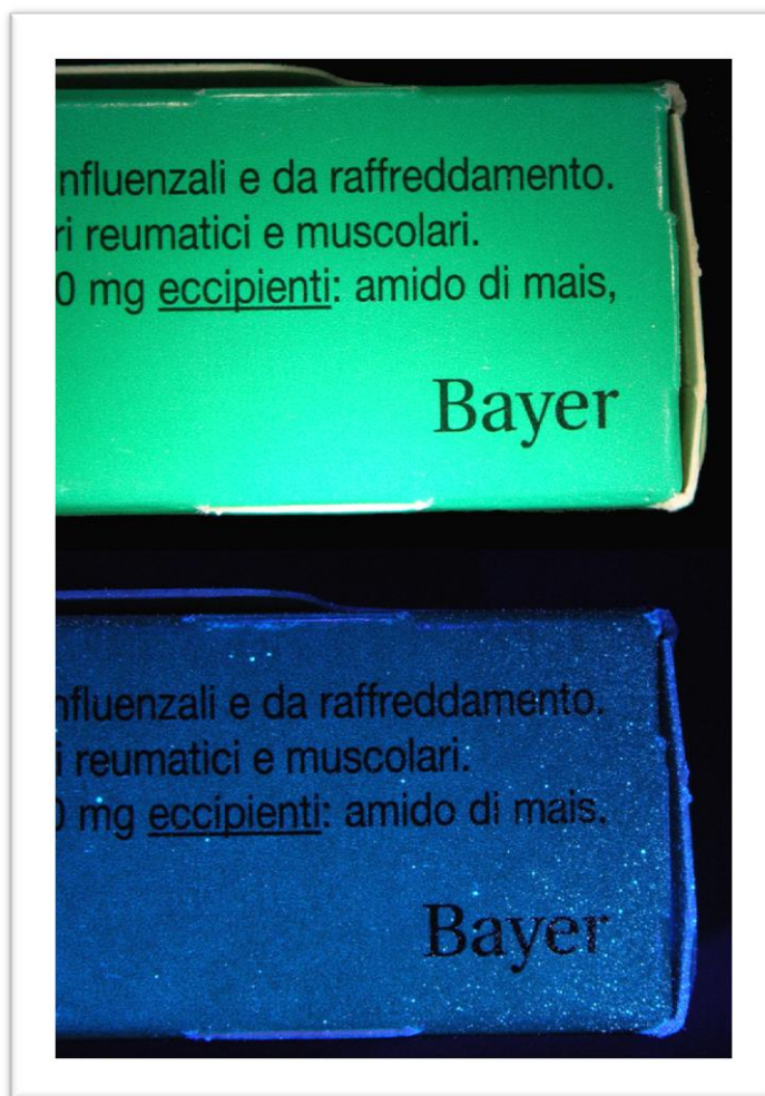
Figure 4.25 – In (a), Drug package under white light illumination is shown, while in (b) the same package is acquired under UV illumination, showing the speckle pattern.
