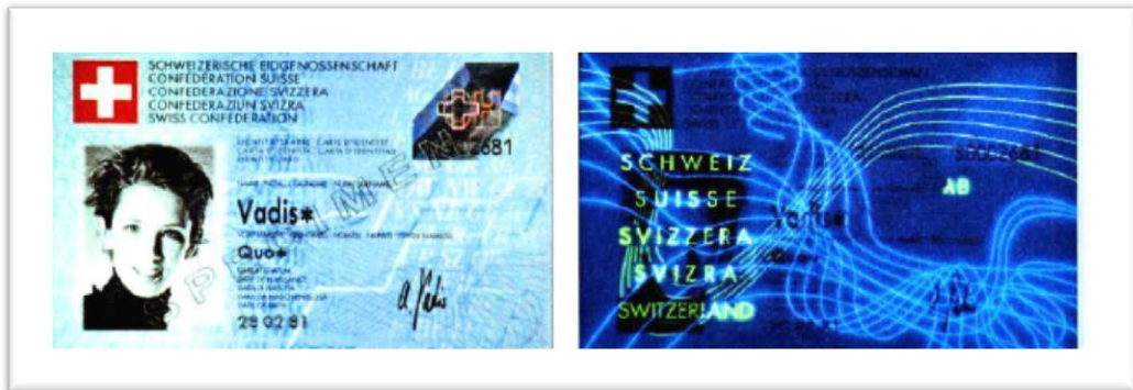
Figure 2.12 – The fluorescent overprint is often positioned over the biographical entries, to help recognition of spot manipulations. Here a photo of the Swiss ID card in daylight (left) and under UV-lighting (right).
