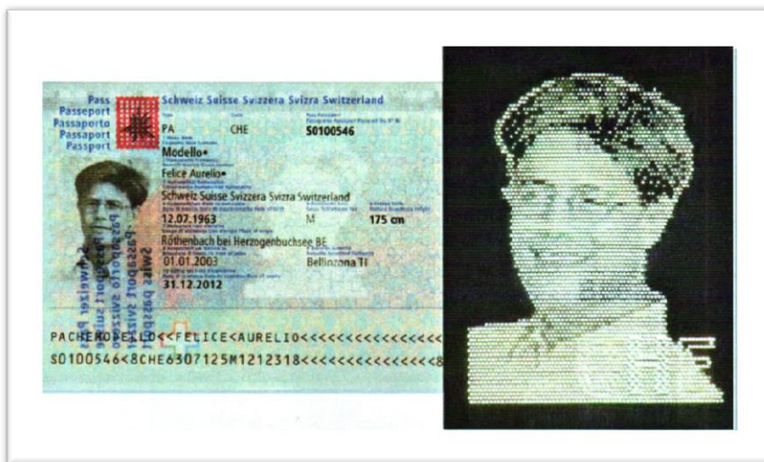
Figure 2.17 – The perforated image is a very sophisticated security element which is simple to verify in transmitted light. The Swiss passport biographical page in an overview (left) and in a close-up of the ImagePerf TM picture (right) .
