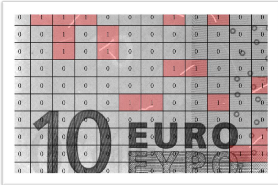
Figure 4.3 – Particular of the same 10 Euro banknote, with superposed a controlling grid. The algorithm assigns a value of 1 to each cell in which is present one or part of a fibre.
