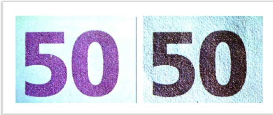
Figure 2.9 – The €50 banknote's denomination figure, printed in OVJ® ink, reflects different colours depending on the angle of the oblique light.
