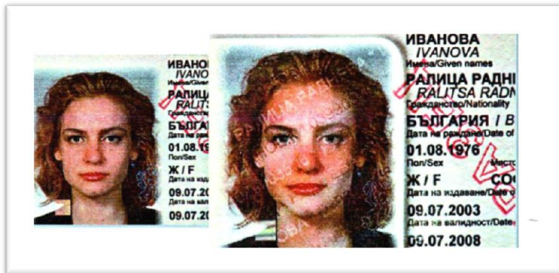
Figure 2.14 – A special digital print allows data to be encoded into an image. Without the use of a special device, the information is not seen (left). Using a decoding lens, the information becomes visible (right)
