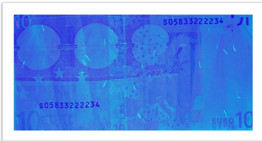
Figure 4.2 – 10 Euro banknote image acquired using UV light source. It is possible to see the random distribution of metallic security fibers.
