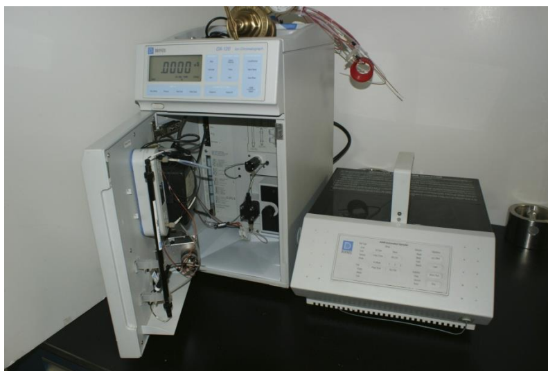
Figure 21 Dionex DX-120 Ion Chromatograph
