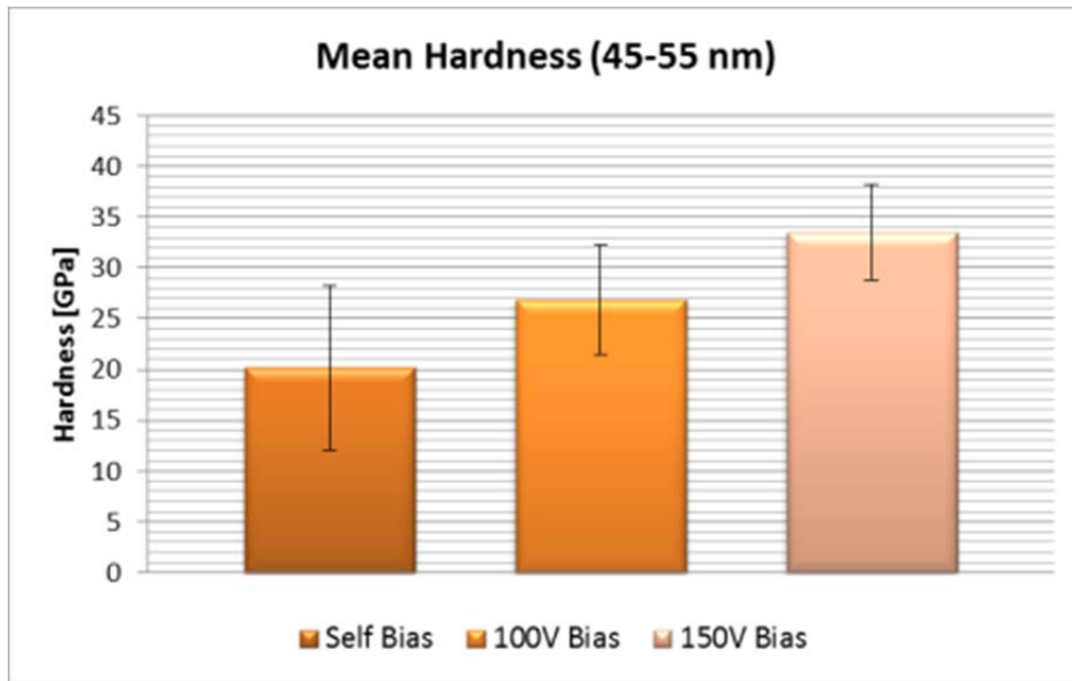
Figura 256: Samples 1852,1860,1866 –75% N 2 , Self Bias, 100V Bias, 150V Bias – Hardness
