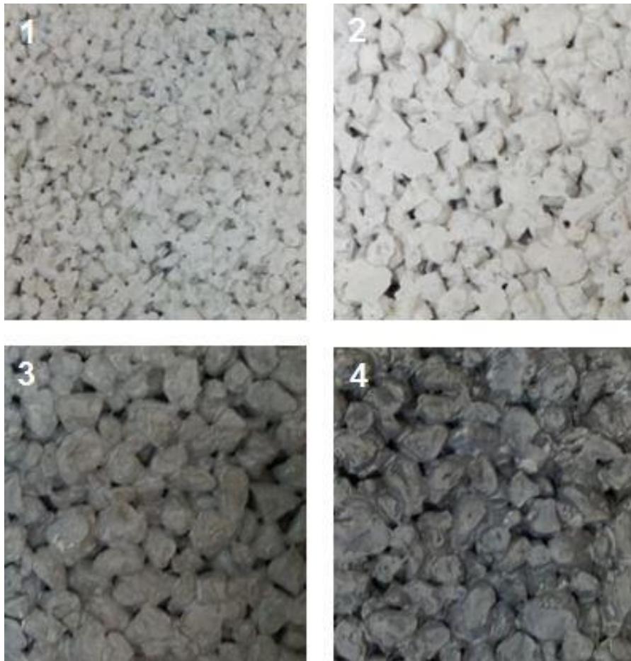
Figure 5.11: Porous concrete samples selected: White Grain Size 6 mm (1), White Grain Size 12 mm (2), Light Grey Grain Size 12 mm (3), Dark Grey Grain Size 12 mm (4).
