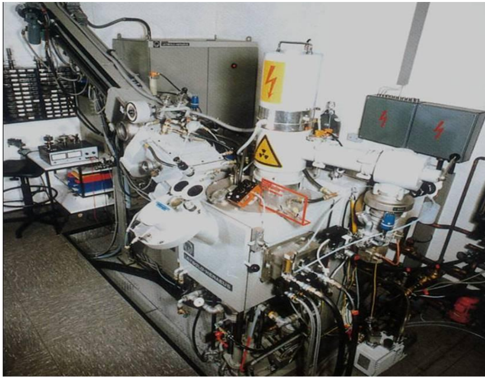
Fig. 3.1: 60 kW LEYBOLD ESC equipment for EV-PVD deposition.
