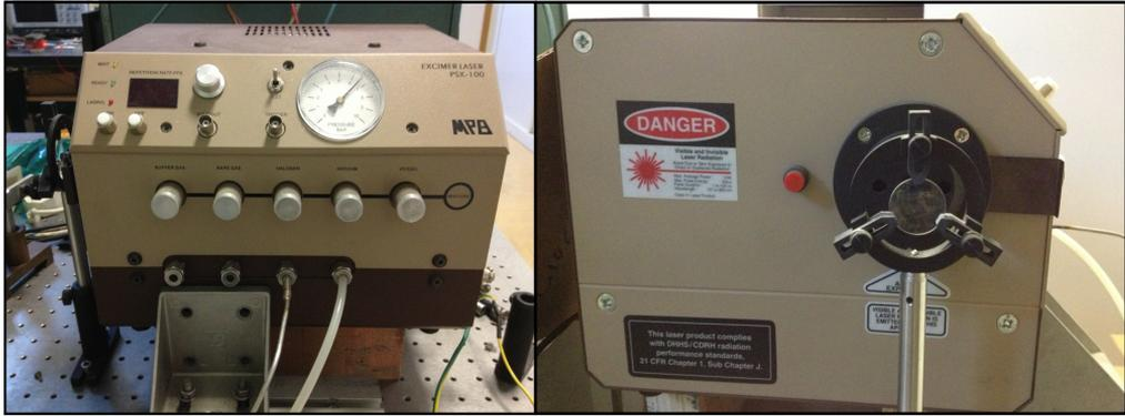
Figura 4 - Neweks PSX100 ArF laser a eccimeri 4.5 mJ/impulso, spot 2x3 mm<sup>2</sup>.
