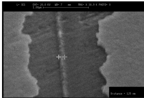
Figure 72 – a 125 nm self aligned gate electrode
