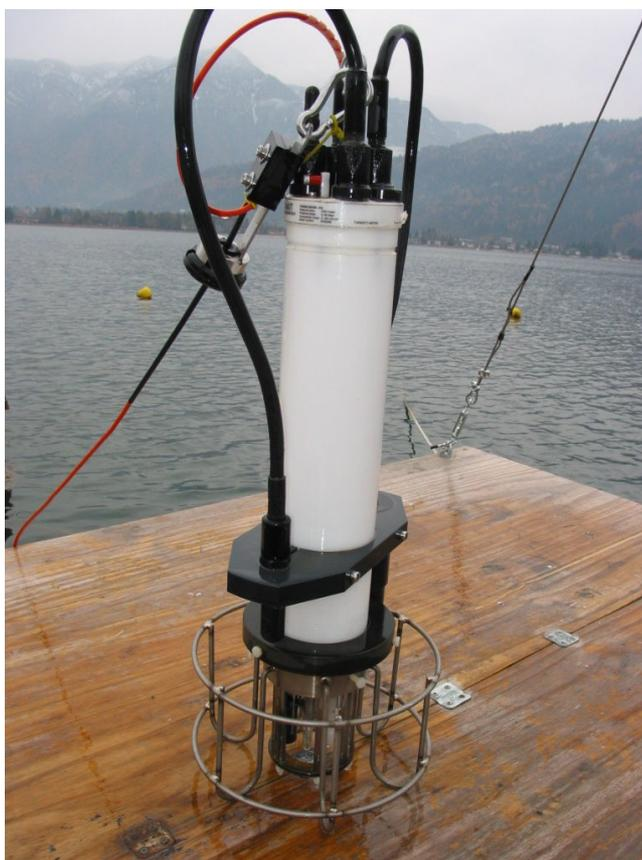
Fig. 2.8. Sonda multiparametrica Idronaut Ocean Seven 316Plus.
