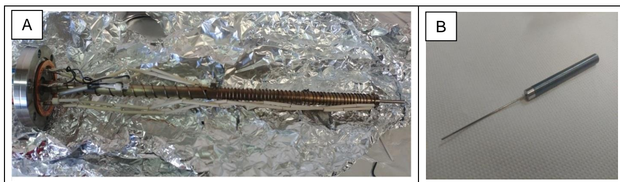
Figure 2.2. Pictures of A) heating system and B) crucible used in time of flight mass spectrometer installed at the CNR-ISM laboratory in Rome.
