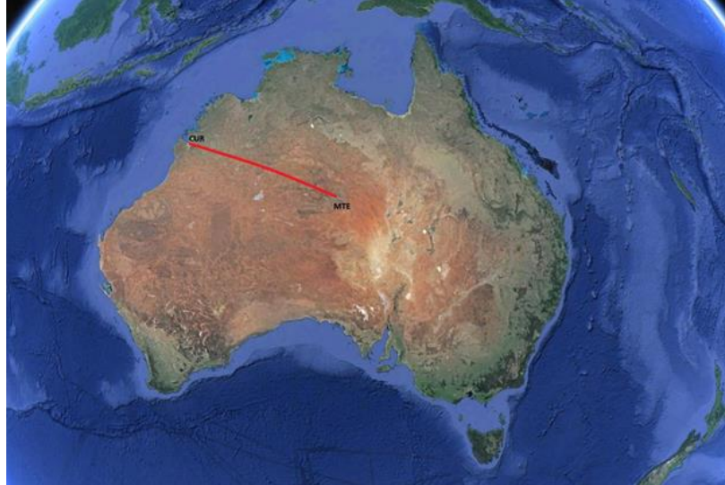
Fig. 6.3. The 1218 km radio-link between the Australian SWS ionospheric stations of CUR (17.60° S; 123.82° E) and MTE (23.52° S; 133.68° E) (red line) (courtesy of Alessandro Ippolito).
