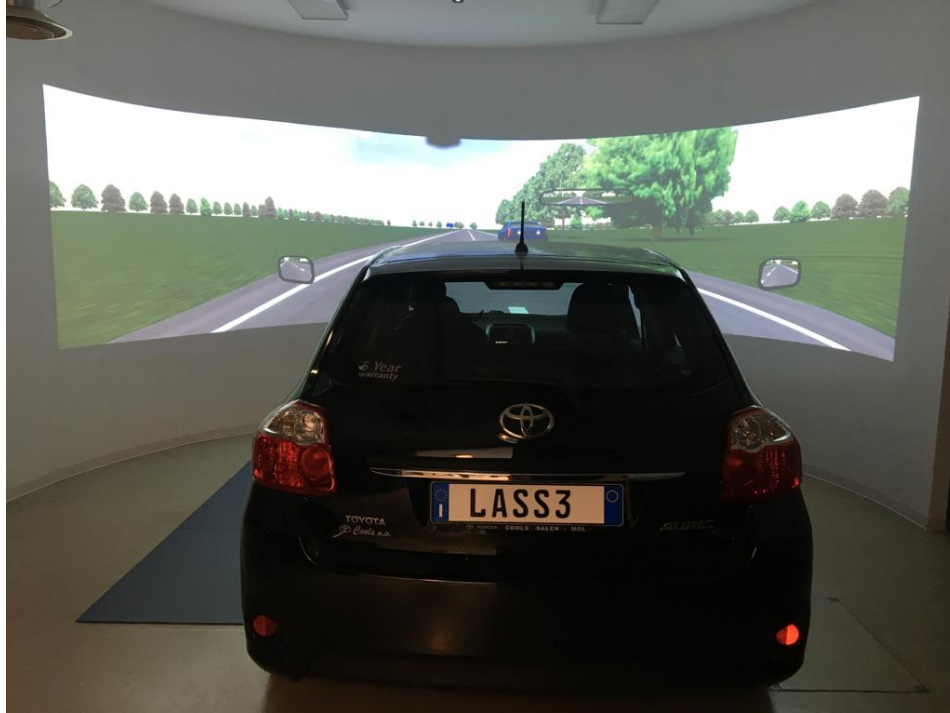
Figure 2.1: Virtual Reality Driving Simulator of Roma Tre University
