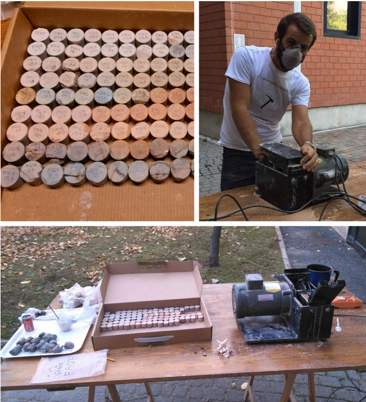
Fig.3.6 Specimens preparation procedure. Cutting process was performed using a double-disc cutting machine, in order to obtain standard cylindrical paleomagnetic specimens around 10,3\text{cm}^3 in volume.
