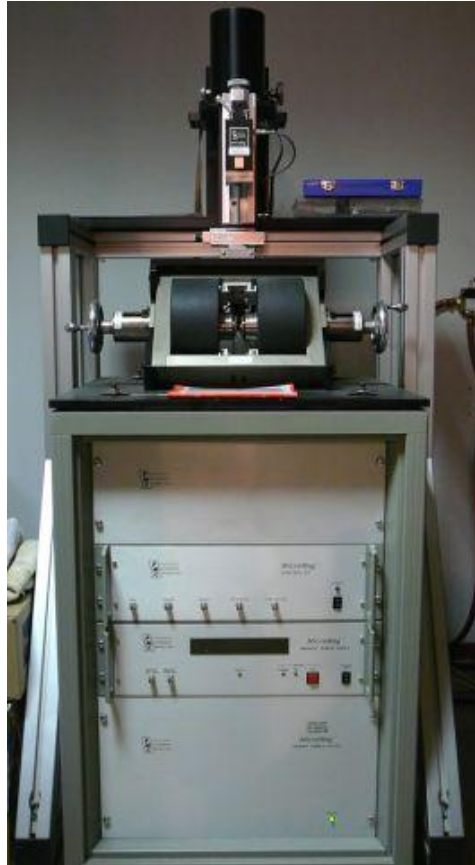
Fig.3.9. Micromag 3900 Vibrating Sample Magnetometer from Princeton Measurement Corp. (USA) available at the Paleomagnetic Laboratory of the INGV. Used to perform IRM acquisition curves, backfield curves and hysteresis loops in powdered samples
