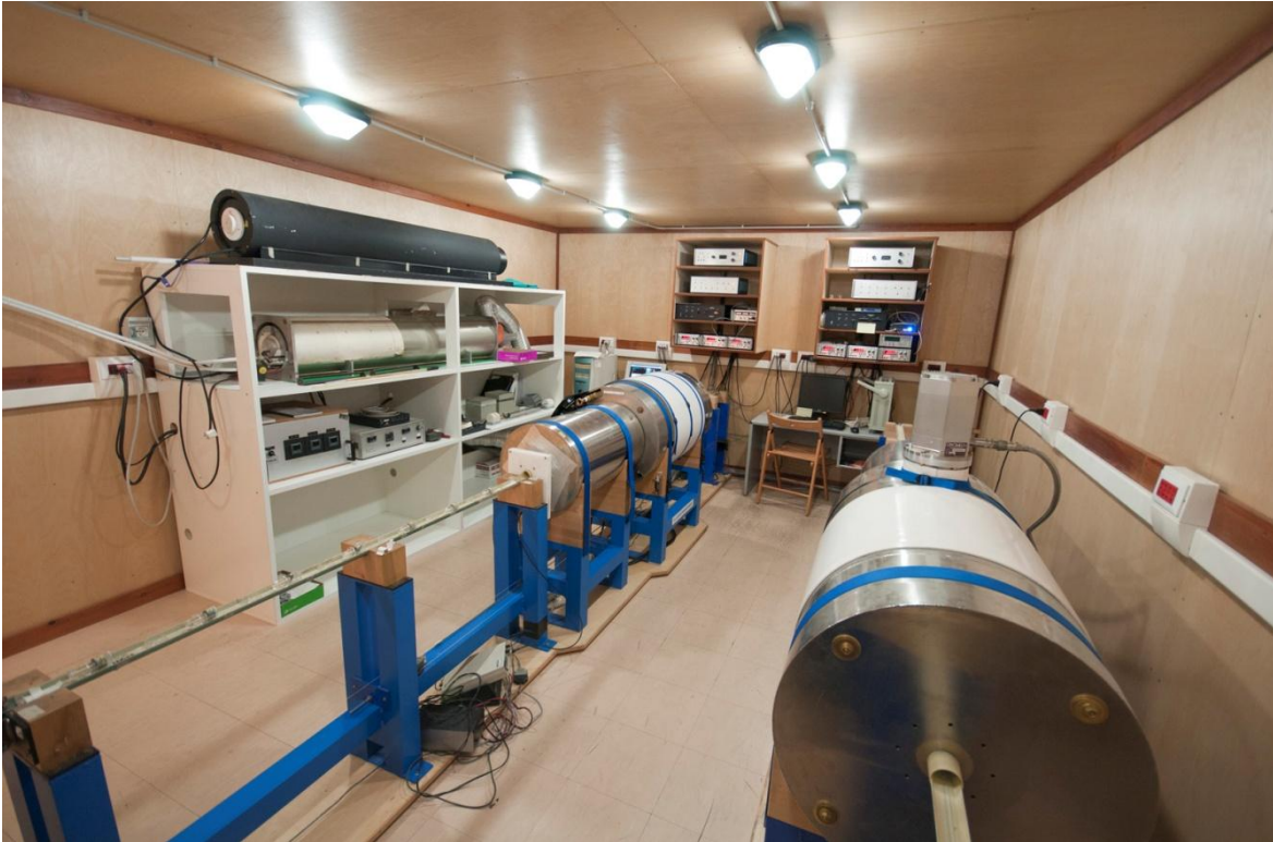
Fig.3.12. DC-SQUID cryogenic magnetometers from 2G Enterprises at the Laboratory of Paleomagnetism of the INGV-Rome Institute. Two Cryogenic magnetometers are installed in a shielded room.
