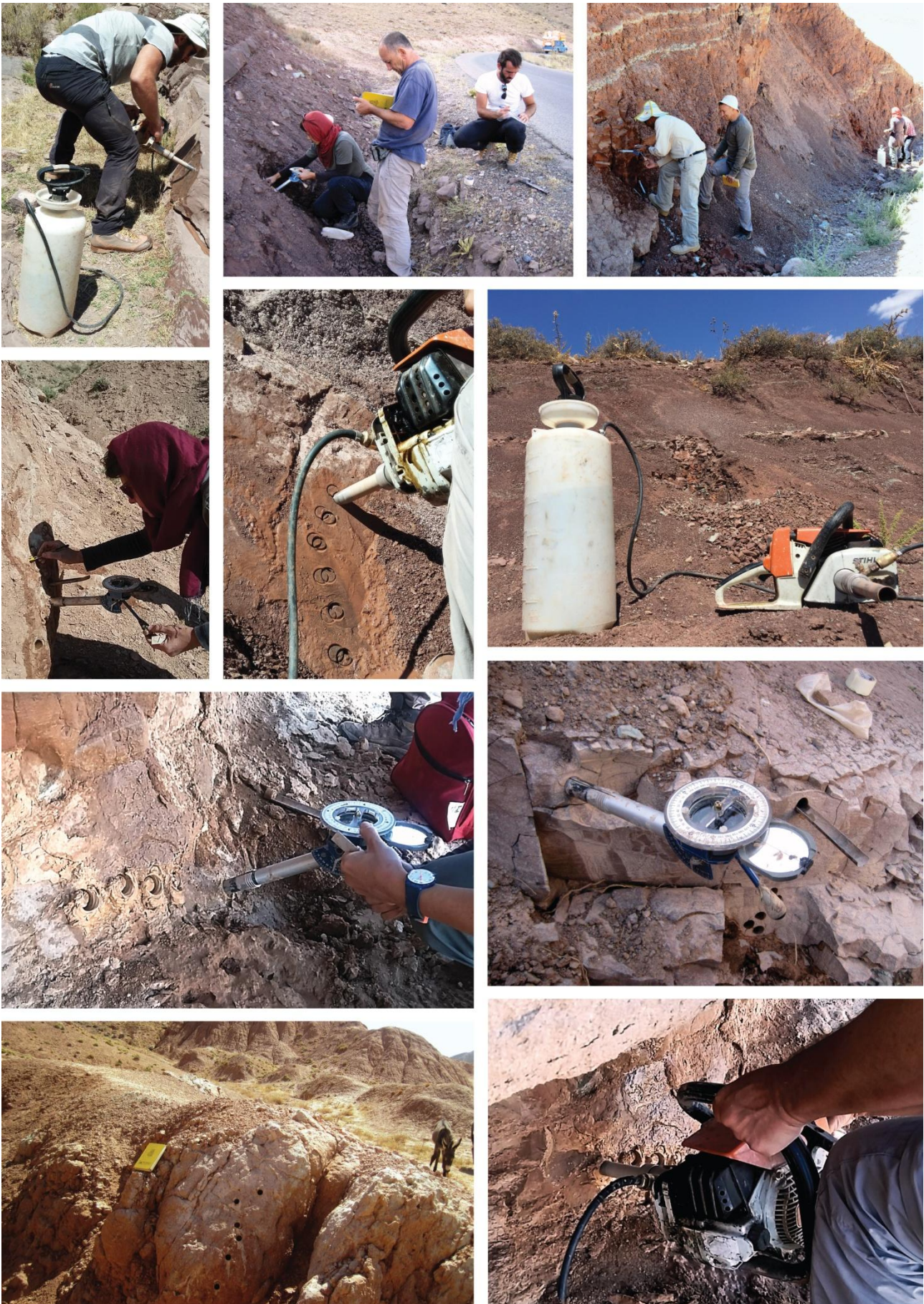
Fig.3.4 Core sample collection procedure. Sampling techniques include the use of a gas-powered drill machine with diamond drilling bit. Cores are signed and oriented in situ with an inclinometer attached to a compass.
