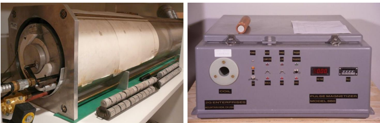
Fig.3.8. This model of paleomagnetic oven shows two differentiated compartments that allow to simultaneously heat and cool two groups of samples. Around 45 samples can be processed in one compartment.
