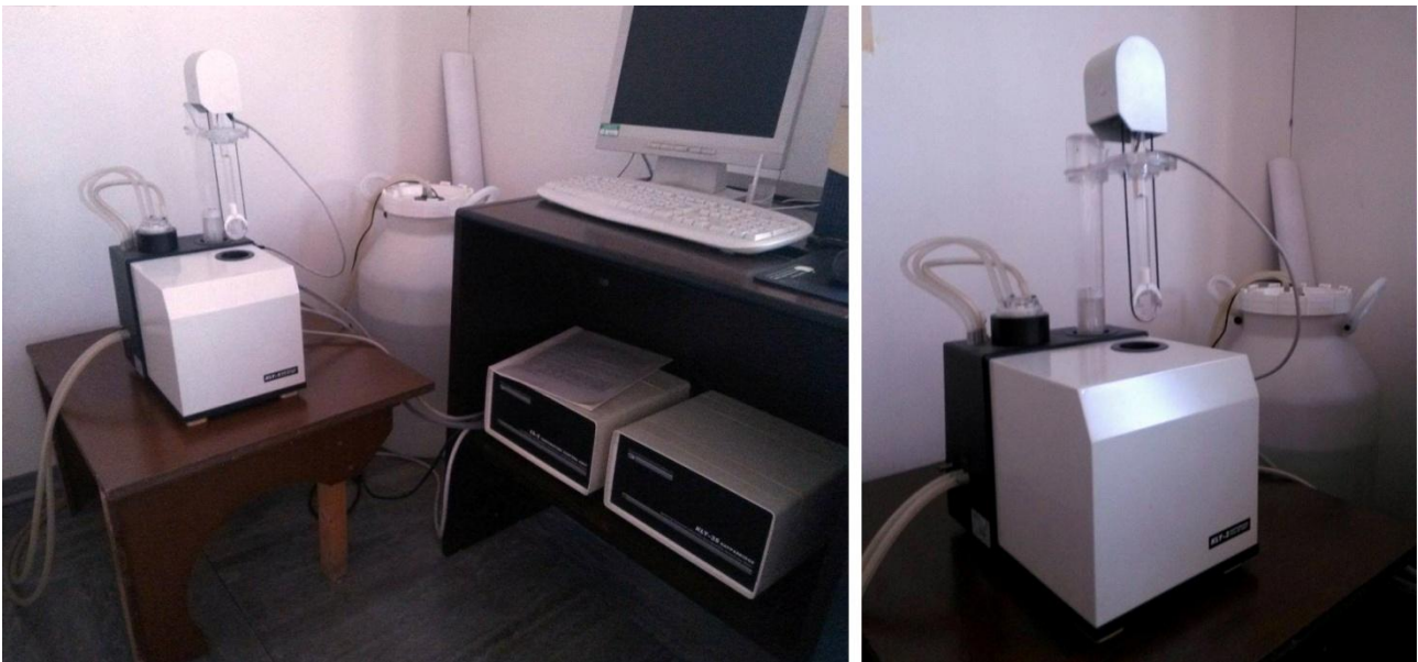
Fig.3.11. KLY-3S Kappabridge susceptometer from AGICO Inc. (Czech Republic) available at the Paleomagnetism Laboratory of the University of Roma Tre.
