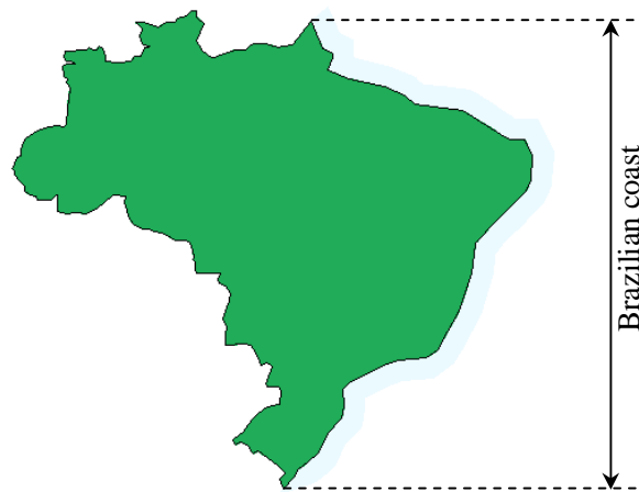
Figure 3.01 Brazilian coast: considered aggressive environment for reinforced concrete structures
