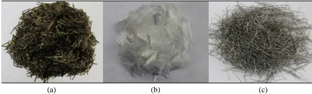
Figure 6.01 (a) Basalt micro-fiber; (b) Polyethylene micro-fiber; (c) Hooked Stainless Steel fiber
