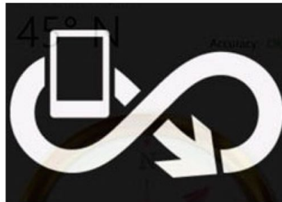
Figure 1: Movement as Möbius strip for the magnetometer calibration.
