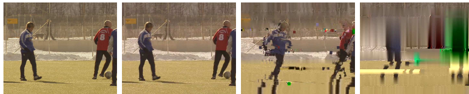
Figure 5.3: Visual impact of different jitter. From left to right: original frame, 1 ms (PSNR 30.67 dB), 2 ms (PSNR 14.75 dB), and 5 ms (PSNR 13.07 dB).
