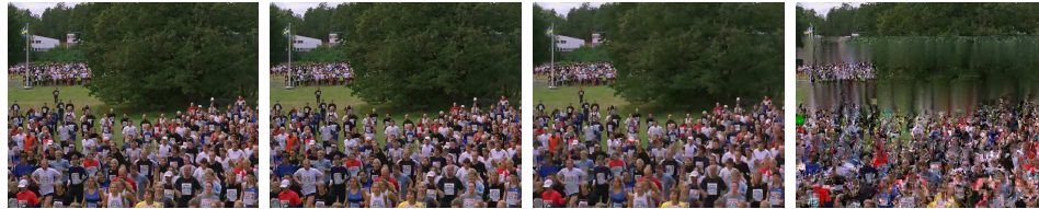
Figure 5.4: Visual impact of PLR. From left to right: original frame, 0.1 % (PSNR 25.03 dB), 1% (PSNR 22.30 dB), and 10% (PSNR 13.90 dB).
