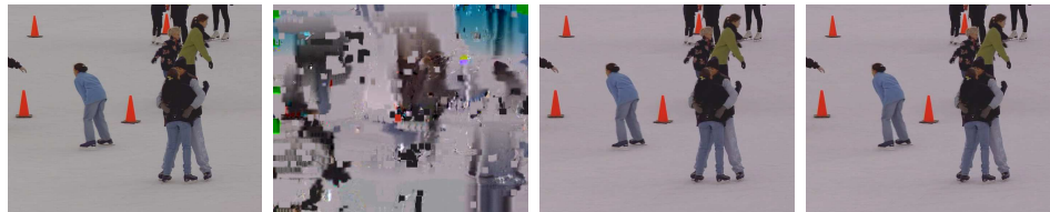
Figure 5.7: Visual impact of different bandwidth limitation. From left to right: original frame, 0.5 Mbps (PSNR 10.54 dB), 2 Mbps (PSNR 33.18dB), and 5 Mbps (PSNR 33.18 dB).
