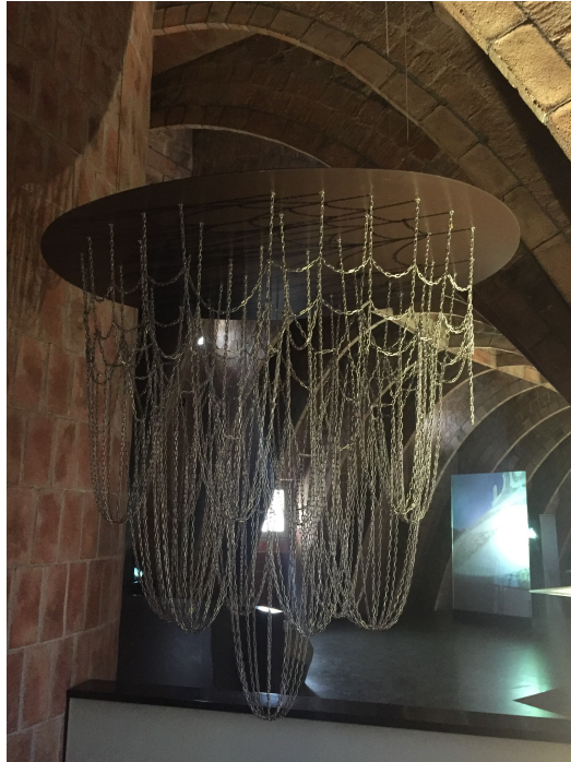
Figure 3.5: Reproduction of Gaudi's chain model displayed at the Casa Milà or Pedrera, Barcelona [PC: Author]
