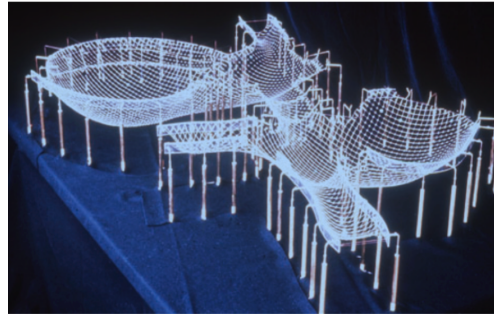
(b) Chain model for the Mannheim Multihalle (Germany, 1974) [Image in the public domain]
