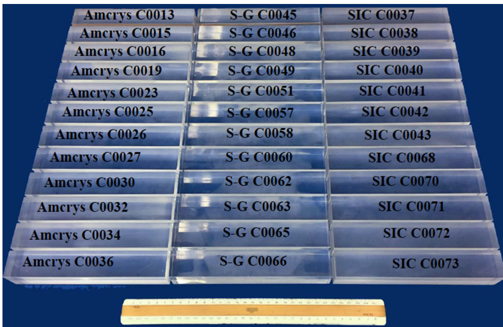
Figure 4.1: Picture of the pre-production crystals received from Amcrlys, Saint Gobain and Siccas vendors.
