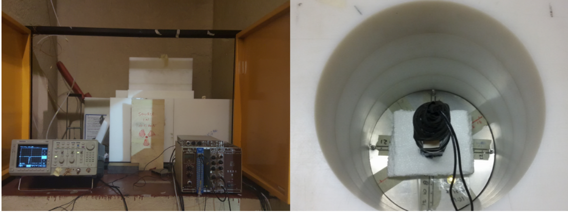
Figure 4.21: Experimental setup used to determine crystal neutron RIN.
