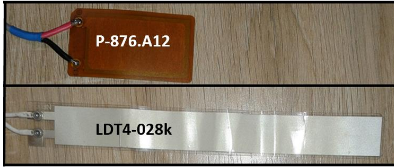
Figure 6D. The P-876.A12 transducer [144] and the LDT4-028k transducer [145].
