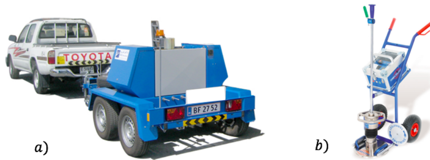
Figure 1.15: Typical configurations of a) FWD and b) LFWD
