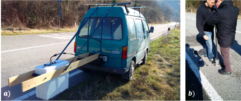
Figure 2.5: The GPR (a) and LWFD (b) equipment utilised for surveys in Rieti (IT), 2014
