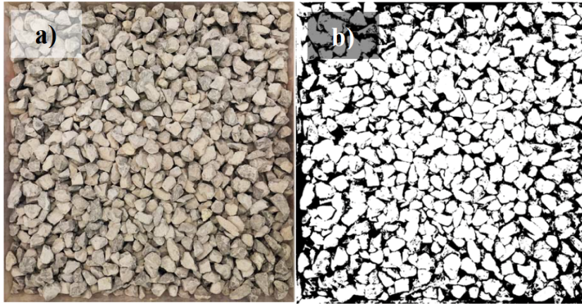
Figure 4.7: Plan view of the ballast-filled methacrylate tank, from Test 1. (a): the raw picture taken with a photocamera suspended in the air above the center of the formwork. (b): the binary image obtained from the processing of the raw picture.
