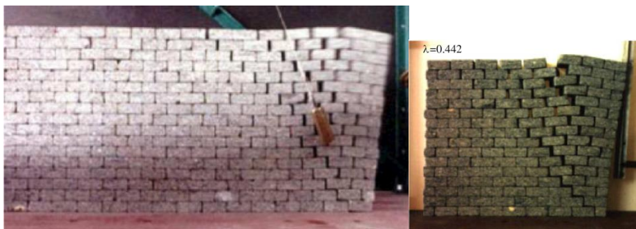
Figure 3.5 Experimental analysis for r=0.5 (left) and r=1 (right), texture B.
