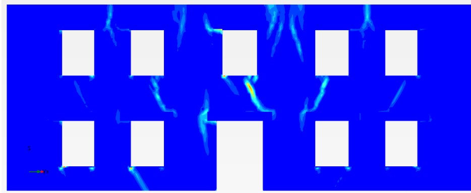
Figure 4.69 Rear façade damage.
