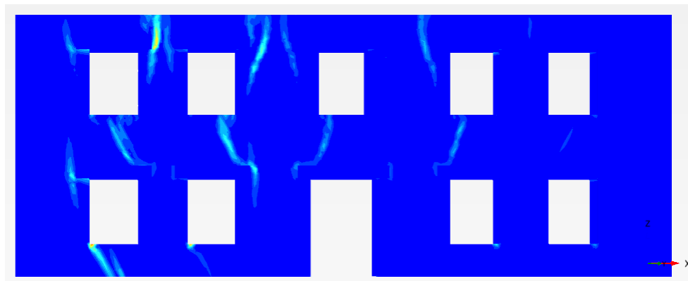
Figure 4.68 Front façade damage.
