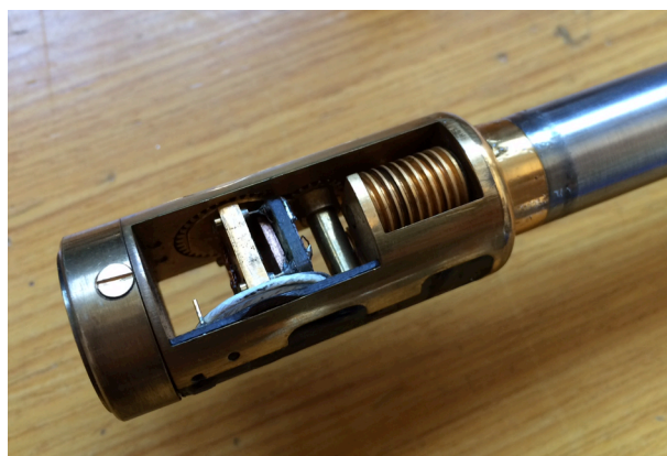
Fig. 3.3. A photograph of the sample holder used in the DC transport measurements.
