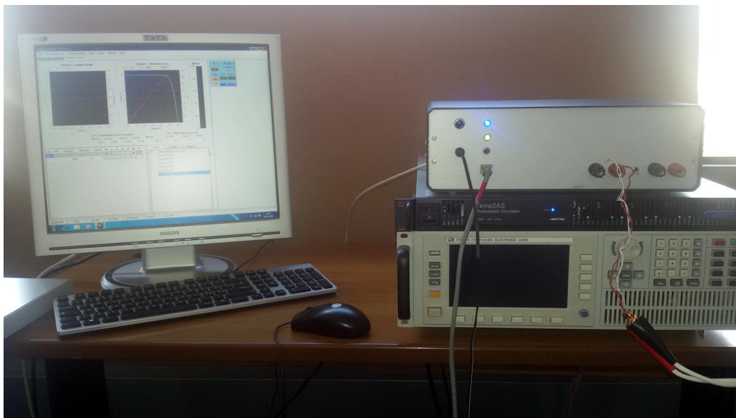
Figure 3.3: Experimental setup used to test the system. On the top there is our system, below it the PV panel simulator Elgar ETS TerraSAS ETS60X14C
