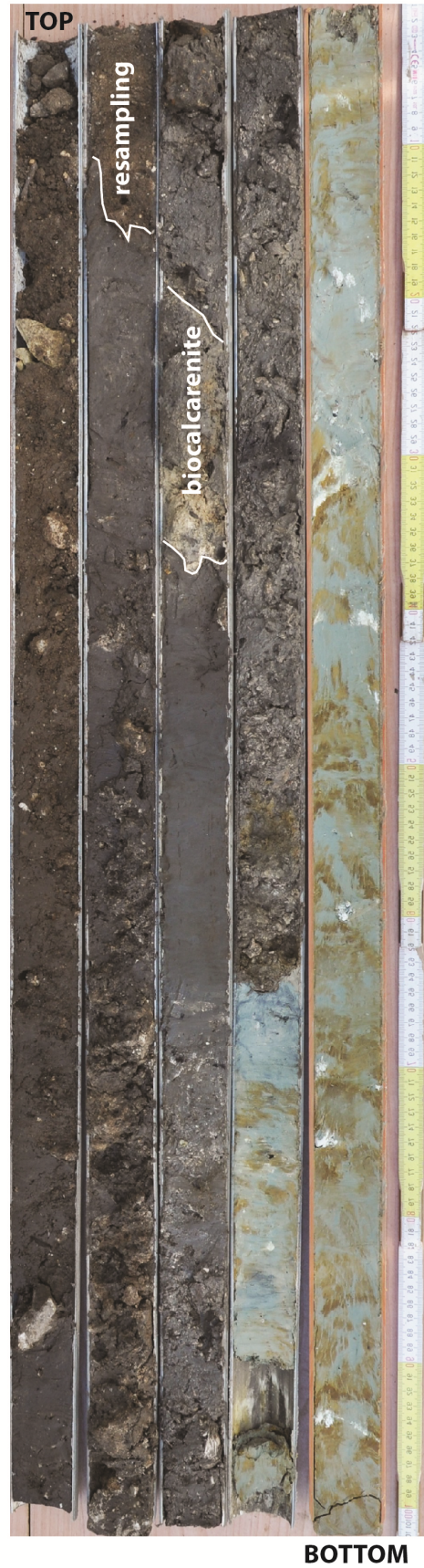
Fig. 13 - SSV-S3 core log with a brief paleoenvironmental reconstruction based on micropaleontological analysis and 14C calibrated ages. On the right, a picture of the whole collected sequence with PVC tubes, 1 m long.
