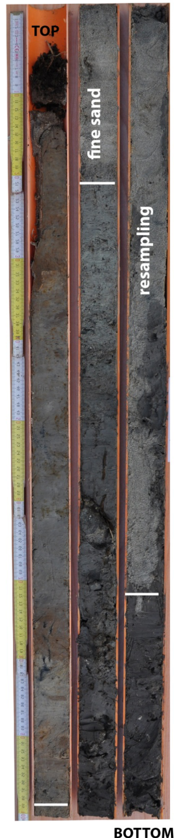
Fig. 8 - VBG-S5 log within a brief paleoenvironmental reconstruction based on micropaleontological analysis and the age result of a radiocarbon dating that constrain the whole sedimentary core sequence. On the right, the picture of the whole collected sequence with PVC tubes, 1 m long. In the core picture the presence of the sandy unit and of a thick resampling interval are highlighted.
