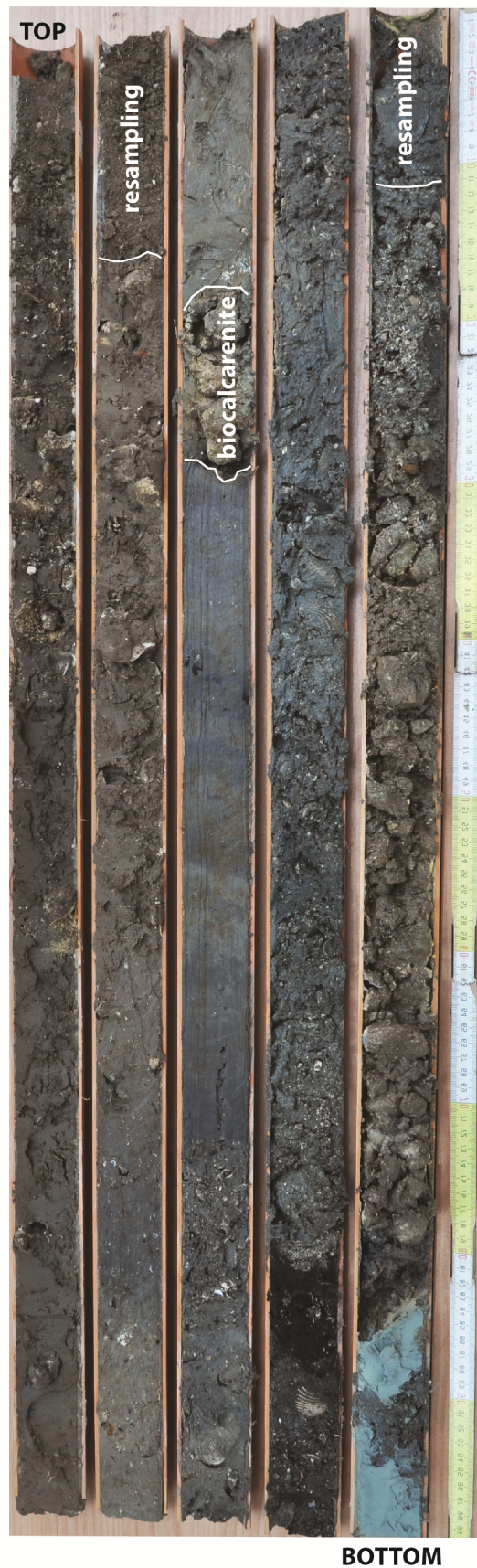
Fig. 12 – SSV-S2 core log with a brief paleoenvironmental reconstruction based on micropaleontological analysis and 14C calibrated ages. On the right, a picture of the whole collected sequence with PVC tubes, 1 m long.
