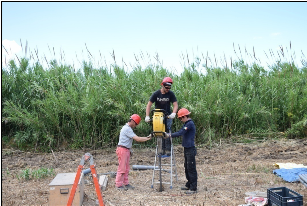
Fig. 2 -The figure shows one of the several steps characterizing the extraction core-procedure. In detail, the operator drives the corer into the ground through the use of the percussion hammer.
